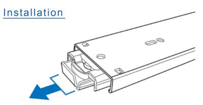
(Pull the center slide all the way out until it reaches the end)
