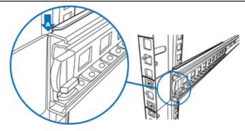
Aline front outter rail to the indent of L bracket between Point A & B.
