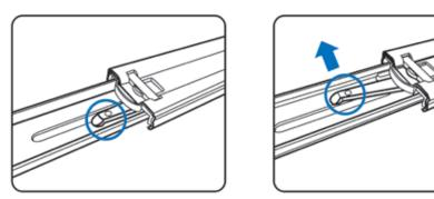
You will see a locking clip at the end point of the center slide. Push it down and unlock the center slide.
