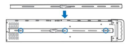
Now put the center slide right next to the rackmount chassis. You should be able to find screw holdes on both sides of chassis. Holes are used for mounting the center slide. Later, the center slide will be use for attaching the sliding rail.
